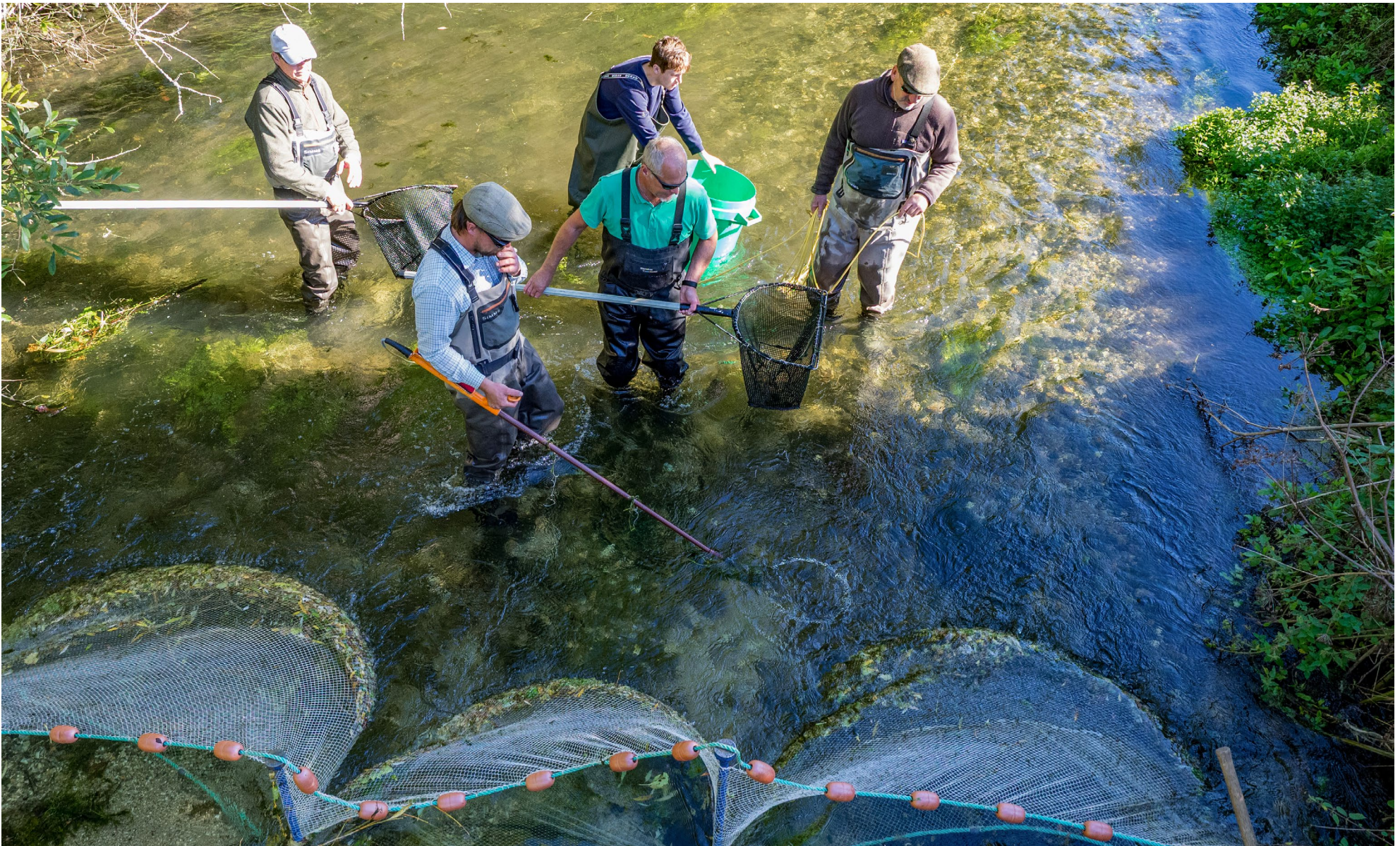
The photo shows the stop nets at the top of the stretch. One operator is holding the insulated orange handle of the anode, two are netting fish, one is managing the holding bin and another holds the yellow power cord from the generator, which on this occasion is on the riverbank (out of view downstream).
